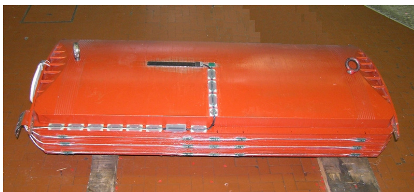
Figure 2. Air Gap Sensors installed at Stator (left) and rotor pole (right)
